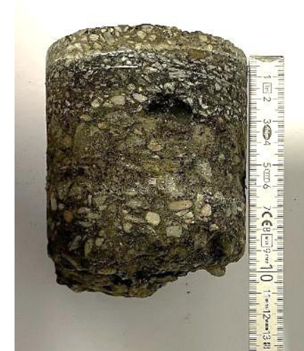
Abb. 31: Bohrkern BK 12 (Dicke = 10 cm)
