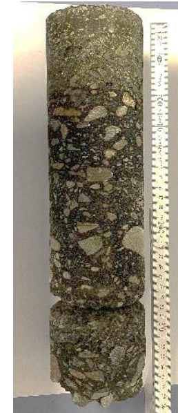
Abb. 4: Bohrkern BK 2 (Dicke = 35 cm)
