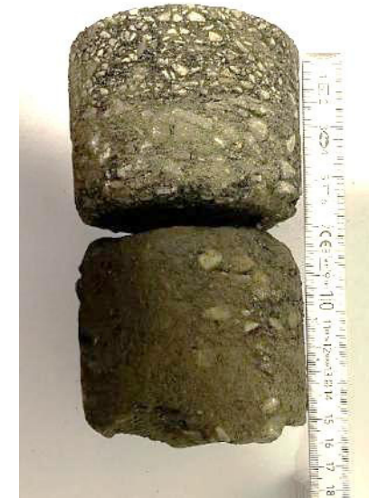
Abb. 23: Bohrkern BK 9 (Dicke = 15 cm)
