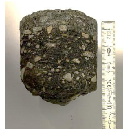
Abb. 26: Bohrkern BK 10 (Dicke = 9 cm)
