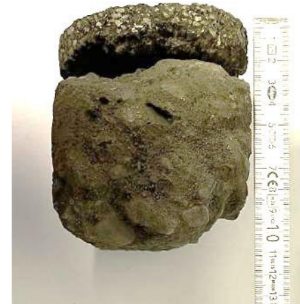
Abb. 12: Bohrkern BK 5 (Dicke = 10 cm)
